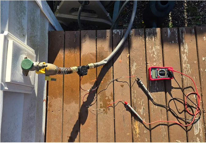
Figure 1. Experimental setup showing the 12 V micro-hydro turbine generator connected to a household hose bib through a threaded adapter, with output measured using a digital multimeter, test leads, and insulated jumper wires.
