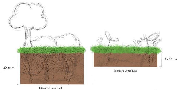
Figure 2. Comparison of intensive and extensive green roof systems based on substrate depth, vegetation type, and structural requirements. Intensive green roofs (left) are characterized by deeper substrate layers (>20 cm), allowing for larger vegetation such as shrubs and trees, increased carbon storage, and enhanced thermal insulation (21). Extensive green roofs (right) have shallower substrate depths (2–20 cm), supporting low-maintenance vegetation such as grasses and sedums, with reduced structural load but lower carbon sequestration and insulation capacity (20). Created by Author (2025).
