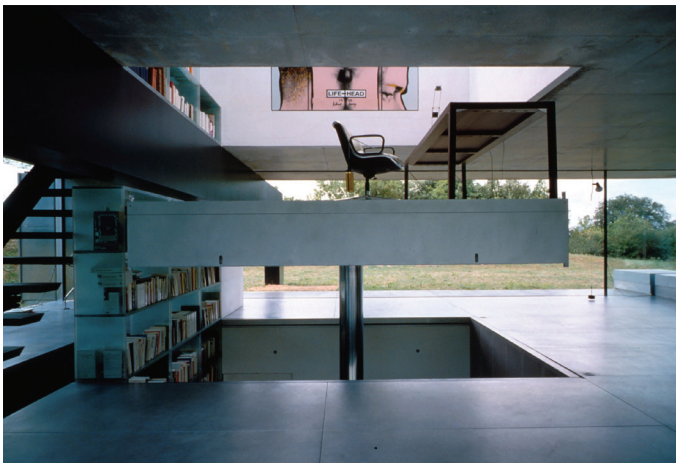
Figure 3. Maison Bordeaux, France. Designed by Rem Koolhaas and OMA in 1998, Maison Bordeaux was commissioned by a client who became paralyzed after a car accident. At its core is a hydraulic platform that moves between three floors, functioning as both circulation and flexible living space. The platform, shifting between roles as study, terrace, or room divider, grants the client spatial freedom and control. This design transforms accessibility into a profound architectural statement on dignity and agency. The figure is reproduced from Reference 16.
