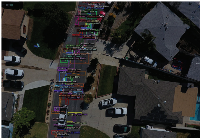
Figure 5. The Sample of Road Distress Instances Detected for Higher Resolution Image.
